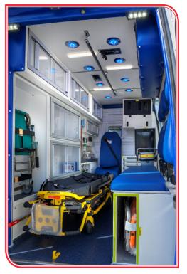
Moisture impervious sub-flooring with high-quality slip-resistant main flooring. Our flooring is
