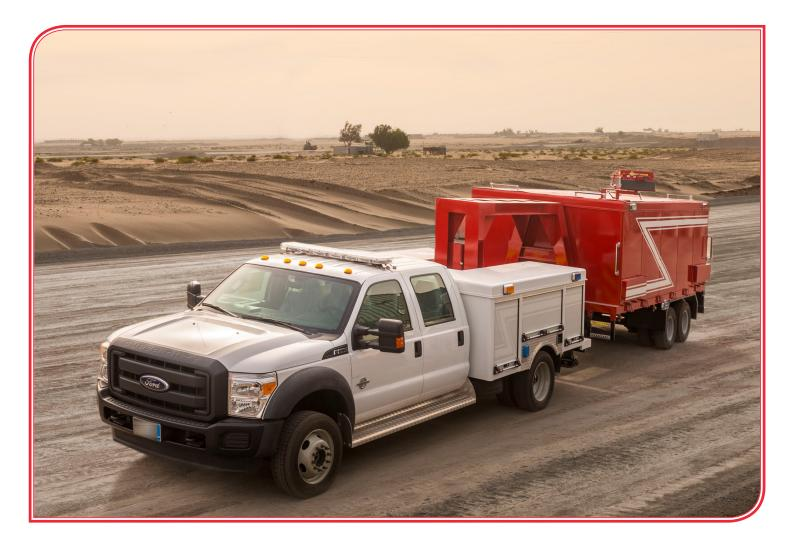
The Fire & Hazard Control (FHC) engineering team has created a versatile combination using the FHC custom built light rescue body and various trailer units. The chassis mounted equipment body and trailer body are all constructed of aluminum using custom designed extrusions for a corrosion free body. The bodies are available in various lengths to accommodate purchaser's equipment and LDH fire hose inventory.
