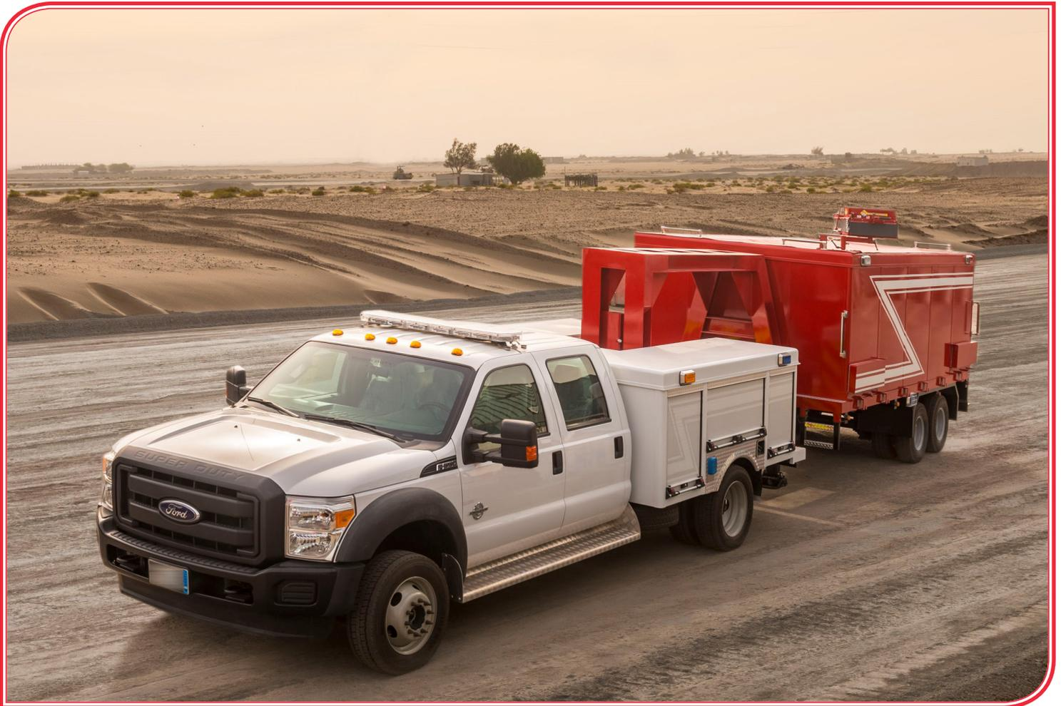
The **Fire & Hazard Control (FHC)** engineering team has created a versatile combination using the **FHC** custom built light rescue body and various trailer units. The chassis mounted equipment body and trailer body are all constructed of aluminum using custom designed extrusions for a corrosion free body. The bodies are available in various lengths to accommodate purchaser's equipment and LDH fire hose inventory.
